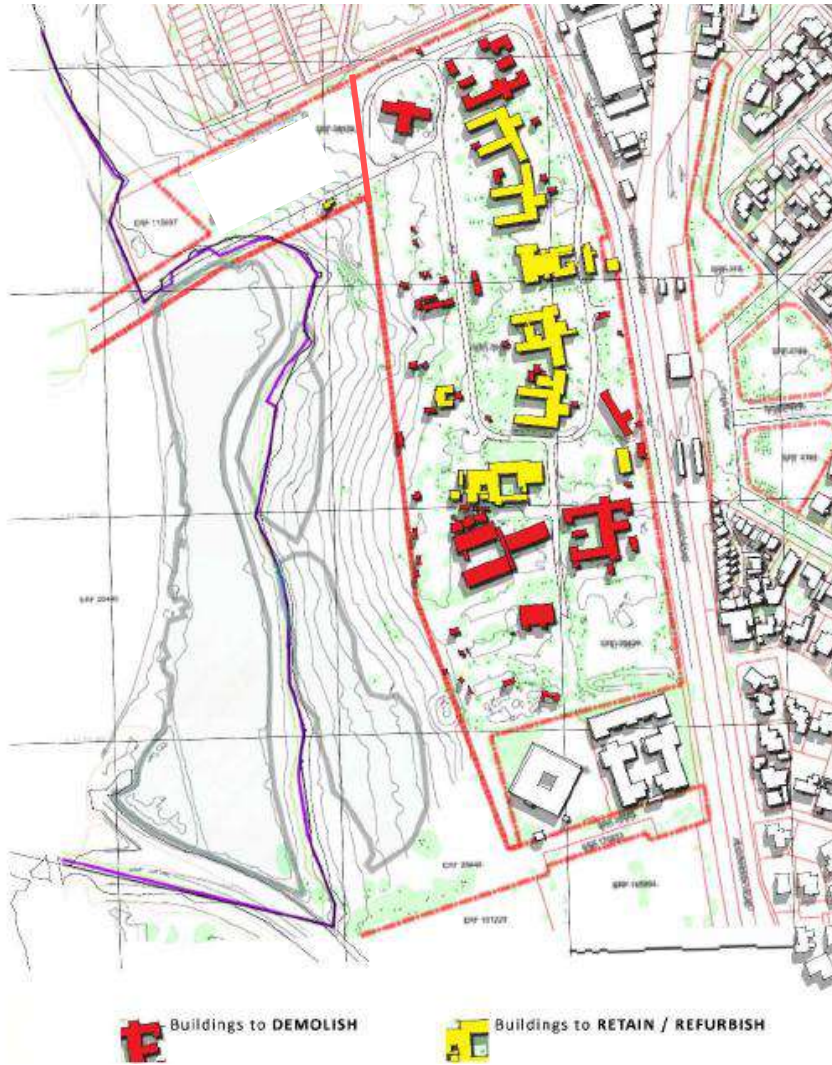
Figure 164: Demolition, retention and refurbishment plan
